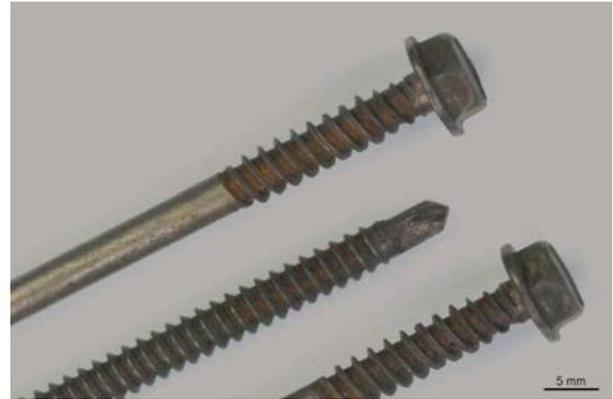
Figure 9: Rolled screws made of 1.4401 with HARD-INOX®-S treatment after a corrosion test according to DIN EN 8442; left: standard treatment, right: adjusted process settings.
